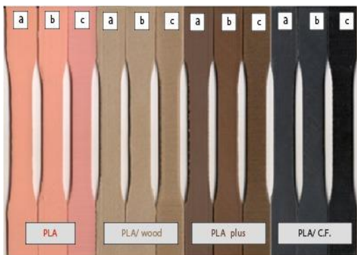
Figure 3. FDM samples of different materials with three-angle orientations: a) Flat, b) On-edge, c) Upright.
