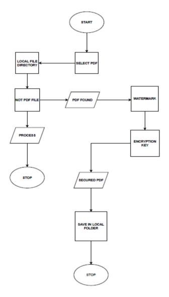
Figure 1. Authentication and Integrity Process flowchart diagram
