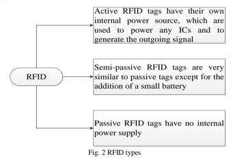
•Passive RFID tags have no internal power supply. The minute electrical current induced in the antenna by the incoming radio frequency signal provides just enough power for the CMOS integrated circuit (IC) in the tag to power up and transmit a response. Most passive tags signal by backscattering the carrier signal from the reader. This means that the antenna has to be designed to both collect powers from the incoming signal and to transmit the outbound backscatter signal.
