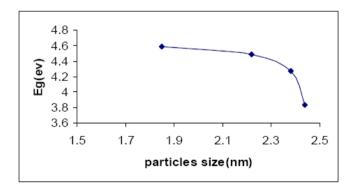
Fig. 4 The variation of particle size with the optical band gap.
