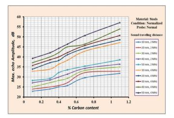
Figure 5. Correlation between Ultrasonic maximum echo amplitude with % carbon content of normalized plain carbon steel samples, using both 2MHz and 4MHz frequencies compression probes.
