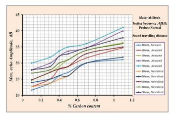
Figure 6. Comparison between annealed and normalized plain carbon steel samples, when carbon content is to estimated ultrasonically using 2MHz frequency compression probes.
