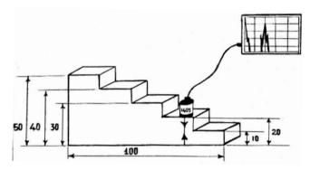
Figure 1. Design dimension of the ultrasonic testing sample, illustrating the normal probe scanning.
