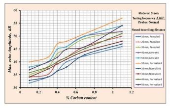
Figure 7. Comparison between annealed and normalized plain carbon steel samples, when carbon content is to estimated ultrasonically using 4 MHz frequency compression probes.
