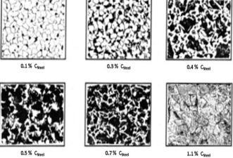
Figure 3. Micrographs representing various carbon steel samples involved in the normalized condition X320.
