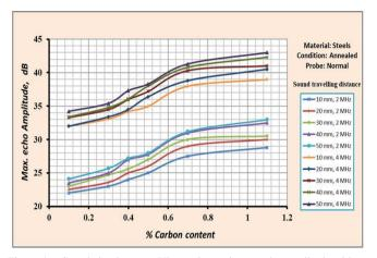
Figure 4. Correlation between Ultrasonic maximum echo amplitude with % carbon content of annealed plain carbon. steel samples, using both 2MHz and 4MHz frequencies compression probes.
