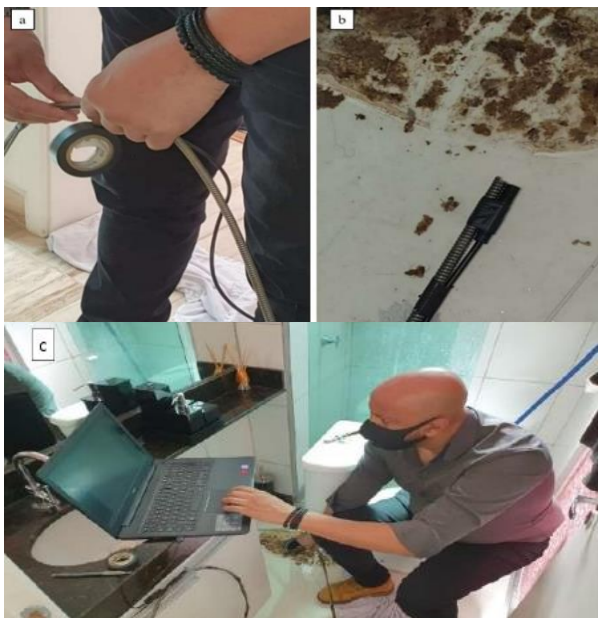
Figure 1. Preparation of equipment for endoscopic evaluation: a) Flexible probe being prepared, b) flexible probe with boroscopes camera, c) probe connected to the computer.
