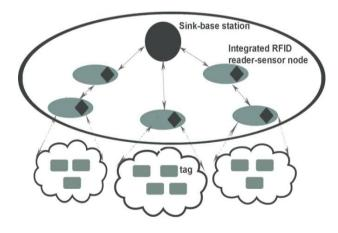
Figure3. Integrating RFID Readers with Wireless Sensor Nodes
