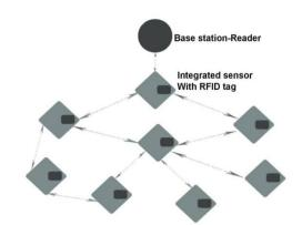
Figure2. Integrated sensor-tags that form a cooperative ad hoc network
