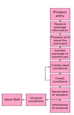
Figure 5. The flowchart of proposed system
