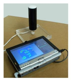
Figure 1. The Hand Grip ForceMap<sup>™</sup> System comprised of a high resolution tactile array sensor mounted to a Delrin<sup>™</sup> cylinder (grip force transducer) that is interfaced to an amplifier/processor and laptop computer.
