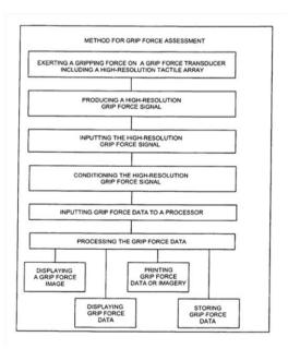
Figure 3. A schematic depicting the steps in involved in the collection and presentation of grip contact force and force distribution via the ForceMap<sup>™</sup> system.
