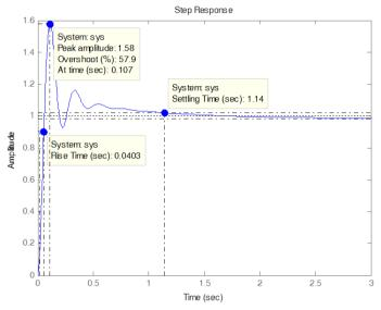
Figure (3): Step response of transfer function (population N.O is 100)
