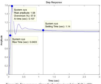
Figure (4): Step response of transfer function (population N.O is 150)
