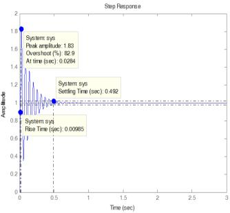
Figure (2): Step response of transfer function (Ziegler - Nichols)
