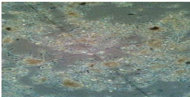
Figure 11. Untreated waste activated sludge at 50x magnification. (Mixture of 20ml sludge and 60 ml water)
