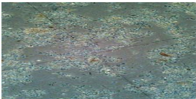
Figure 12. Waste activated sludge treated with ultrasound for 10min at 50 x magnifications. (Mixture of 20ml sludge and 60ml water)
