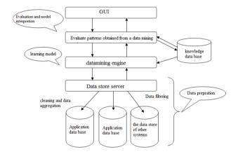
Figure 1. Architecture of a data mining system
