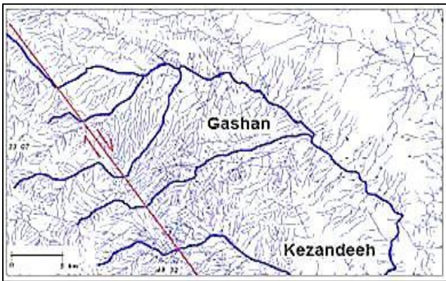
Figure 10. Dextral strike-slip fault along the fault Roudbar (se Gashan villae)
