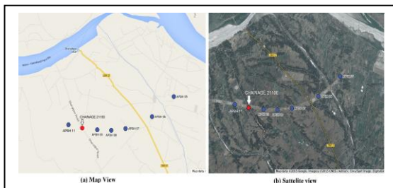
Figure 3. Location of predicted borehole at chainage 21100 (7 Boreholes within chainage 17600 to 21600)
