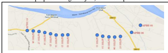
Figure 2. Location of all 15 boreholes within chainage 17600 to 27600 (Jajira Approach Road)
