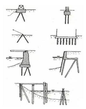
Figure 6. Examples of piles used in onshore and offshore constructions
