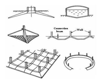
Figure 13. Examples of shell foundations
