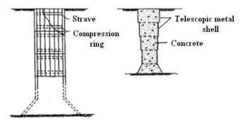
Figure 8. Examples of *in - place* or belled piers [5]
