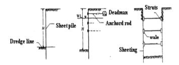
Figure 15. Examples of sheet piling structures [5]
