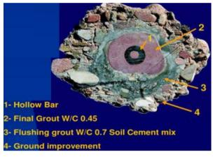
Figure 11. Typical cross section of an exhumed micro pile [7]
