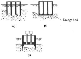
Figure 9. Various types of caisson foundations; a) open, b) box ,c) pneumatic
