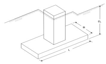
Figure 1. Rectangular single footing [1] *Df* (depth of footing), *B* (width of footing), *L*(length of footing)
