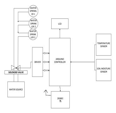
Figure 1. Block Diagram of the System Transmitter
