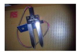
Figure 2. Soil moisture employed for the work
