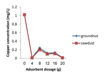
Figure 2. Variation of copper concentration with varying dosages of different adsorbates.
