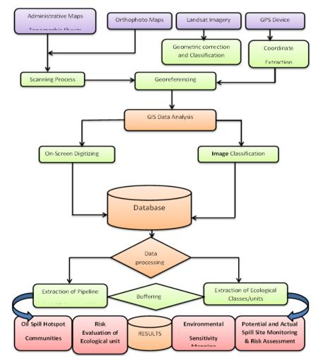
Figure 5. Schematic Diagram of General Data Analysis
