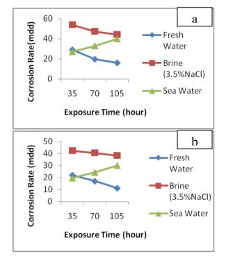
Figure 2. Corrosion rate with exposure time in three different environments. (a) Galvanized CI sheet 1 (b) Galvanized CI sheet 2.
