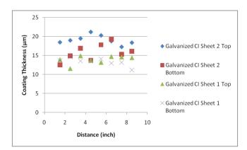
Figure 1. Comparison between the thicknesses of two galvanized CI sheets.
