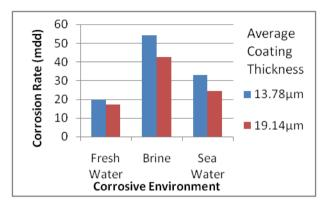
Figure 4. Effect of Coating Thickness on the Corrosion rate of galvanized CI sheets after being exposed in three different environments for 70hours.
