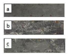
Figure 3. Samples after salt spray test in three different environments for an exposure time of 70 hours. (a) Fresh Water (b) 3.5% NaCl (c) Sea Water.
