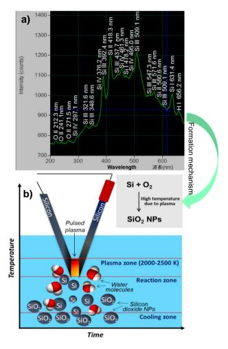
Figure 3. a) Atomic emission spectrum collected form the pulsed plasma discharge zone; b) Formation mechanism of SiO<sub>2</sub> nanoparticles by pulsed plasma in liquid method.
