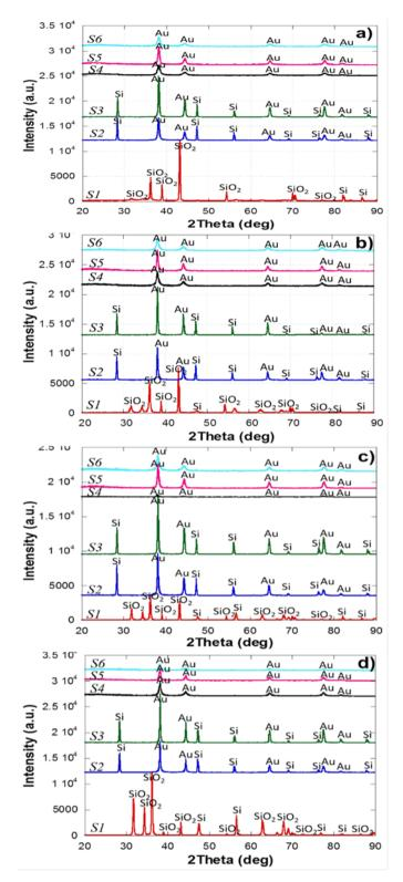
Figure 5. a) XRD pattern for samples obtained right after synthesis, before annealing; b) XRD pattern for samples obtained after annealing at 400 °C, for 2 hours; c) XRD pattern for samples obtained after annealing at 500 °C, for 2 hours; d) XRD pattern for samples obtained after annealing at 600 °C, for 2 hours; d) XRD pattern for samples obtained after annealing at 600 °C, for 2 hours.
