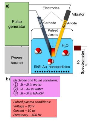
Figure 2. a) Schematics of experimental set up designed for synthesis of  $SiO_2$  and Si-Au nanoparticles by pulsed plasma; b) Electrode and liquid variations with electrical conditions during synthesis.
