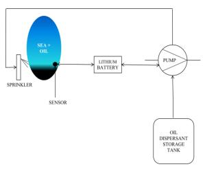
Figure 2. Block diagram of the Automatic Oil Spill Dispeller
