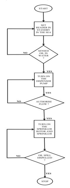
Figure 1. Process Flowchart
