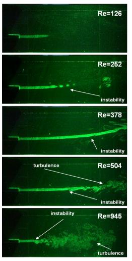
Figure 3. Laminar to Turbulent Transition of a Submerge Jet Flow (Available: http://en.m.wikiversity.org/wiki/Fluid\_Mechanics\_for\_MAP/Introduction)
