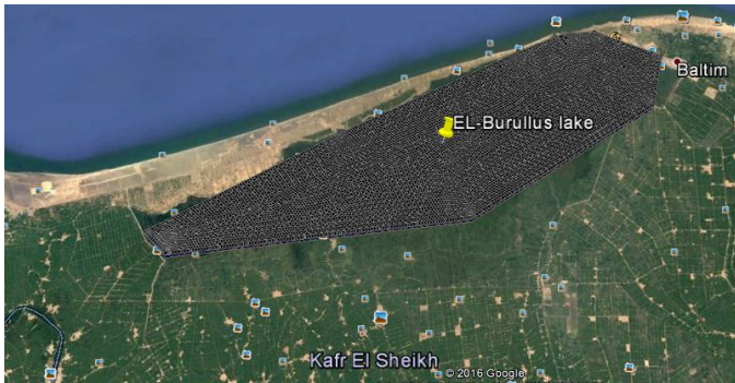
Figure 6. The developed curvilinear grid to discretized Lake El-Burullus.
