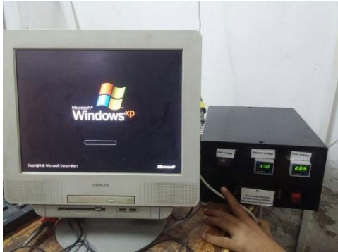
Figure 16. UPQC Working inline with Sensitive Load
