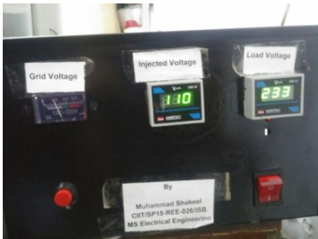
Figure 17. UPQC working at 50% Voltage Sag
