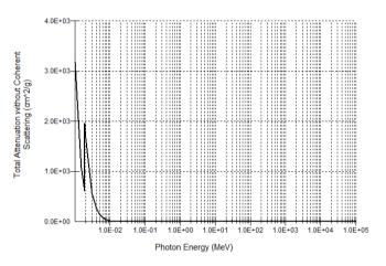
Figure 5. Relationship between total attenuation without coherent and photon energy
