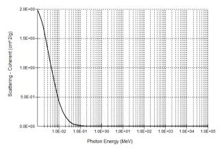
Figure 1. The exponential relationship between scattering – coherent and photon energy.
