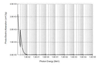
Figure 3. Photon electric absorption of Si versus photon energy
