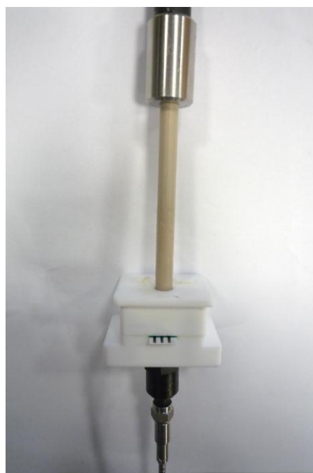
Figure 6. Spectroelectrochemical cell with a fiber from the spectrometer (top) and a fiber that guides the transmitted light to a photomultiplier (bottom). The SPE inside the cell is connected with the potentiostat.
