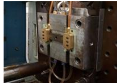
Step 2: heating position (machine induction heating will be turn on)
