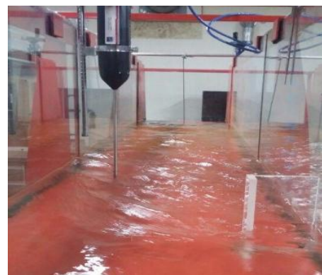
Figure 3. ADV velocimeter during the pickup of velocity components of flow
