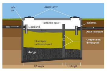
Figure 1. Typical septic tank
