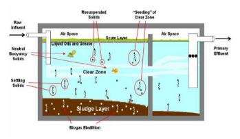
Figure 2. Septic tank processes
