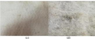
Figure 3. Examined materials (a) Filter labbad (b) Non-woven geo-textile 300 gm (c) Non-woven geo-textile 800 gm (d) Non-woven polyester
