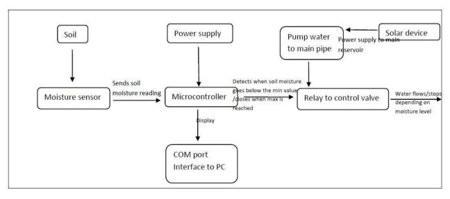
Figure 1. Components of auto watering irrigation system [7]
