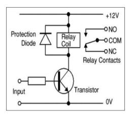
Figure 6. Relay Circuit
