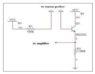
Figure 4. The Schematic Diagram of Humidity Sensor
