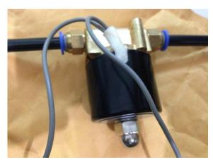
Figure 7. Automated on/off valve
