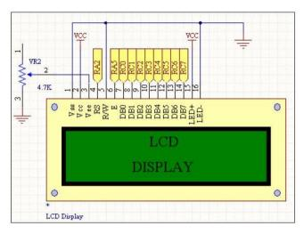
Figure 8. LCD Display Schematic Diagram
