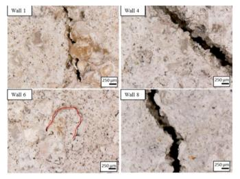
Figure 7. Fissures in the Coating
