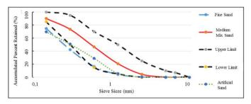
Figure 3. Gradation Curve Fine Sand, Medium Mix Sand and Artificial Sand
