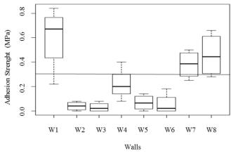
Figure 4. Adhesion results in mortar coating
