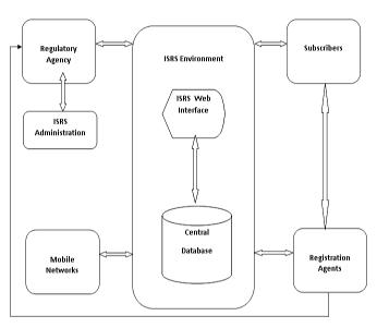
Figure 3. Architectural Design of the Integrated SIM Registration System
