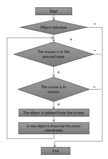
Figure 3. Algorithmic block-diagram of the functional block of object movement
