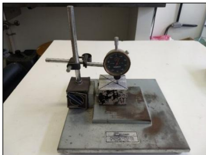
Figure 4. Extensometer used for abrasive wear measuring
