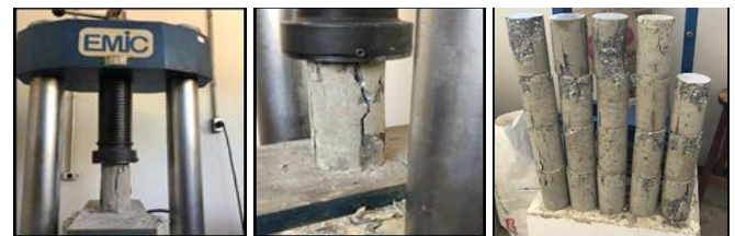
Figure 4. Test specimens ruptured, a, b and c.
