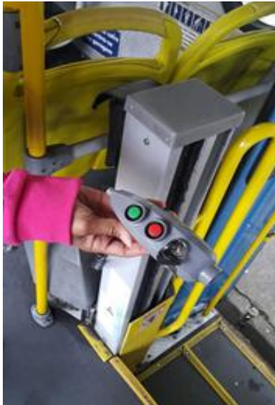
Figure 6. Lift control (source: Author's archive, 2017)
