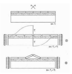
Figure 3. Ceramic coating required by tensile stress, Fiorito (2013)
