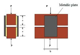
Figure 7. Shear Test - MR-14, RILEM (1993)
