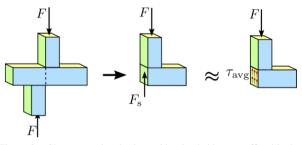
Figure 2. Shear stress in a horizontal bar loaded by two offset blocks, Sanpaz (2009)
