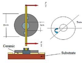
Figure 8. Torsion Test - MR-20, RILEM (1994)
