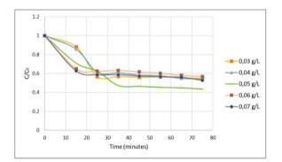
Figure 5. Final concentration by initial concentration of DS  $(C/C_0)$  vs time (minutes). Fixed parameters: NaCl concentration = 1.0 grams per liter, current density = 12 amperes per meter squared, initial pH = 3.
