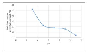
Figure 4. Initial pH of the solution vs. removal of diclofenac sodium (%).
