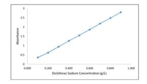
Figure 3. Analytical curve of concentration (in grams per liter) vs absorbance for diclofenac sodium aqueous solutions.
