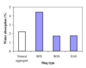
Figure 12. Water absorption of paving blocks containing coarse and fine slag simultaneously
