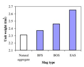
Figure 3. Unit weight of paving blocks containing coarse and fine slag simultaneously
