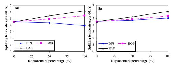
Figure 5. Tensile splitting strength of paving blocks containing, (a) Coarse slag and (b) Fine slag
