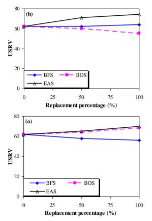
Figure 9. Slip/skid resistance of paving blocks containing, (a) Coarse slag and (b) Fine slag
