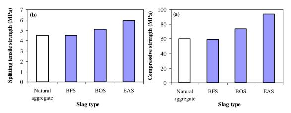
Figure 6. Strengths of paving blocks containing coarse and fine slag simultaneously, (a) Compressive strength and (b) Tensile splitting strength
