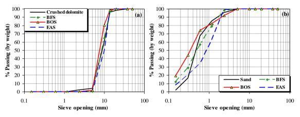
Figure 1. Sieve analysis of aggregates, (a) Coarse aggregate and (b) Fine aggregate
