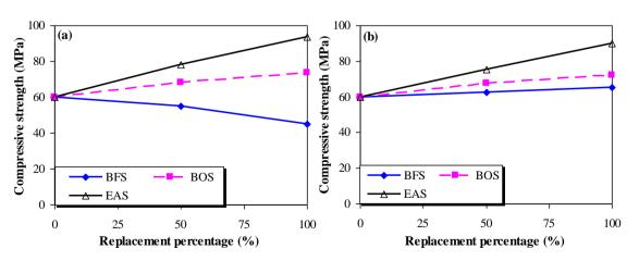
Figure 4. Compressive strength of paving blocks containing, (a) Coarse slag and (b) Fine slag
