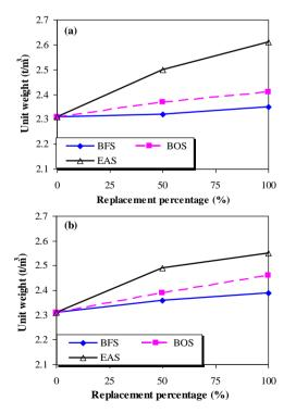
Figure 2. Unit weight of paving blocks containing, (a) Coarse slag and (b) Fine slag
