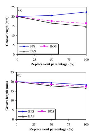
Figure 7. Groove length of paving blocks containing, (a) Coarse slag and (b) Fine slag
