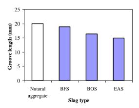
Figure 8. Groove length of paving blocks containing coarse and fine slag simultaneously
