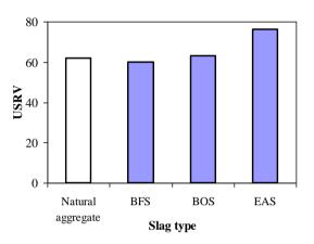
Figure 10. Slip/skid resistance of paving blocks containing coarse and fine slag simultaneously
