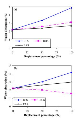
Figure 11. Water absorption of paving blocks containing, (a) Coarse slag and (b) Fine slag
