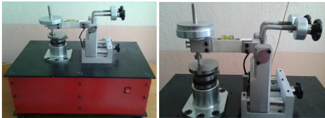
Figure 2. Schematic diagram of wear test machine
