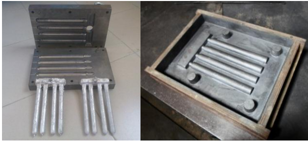
Figure 1. Permanent mold, model plate image for sand mold casting
