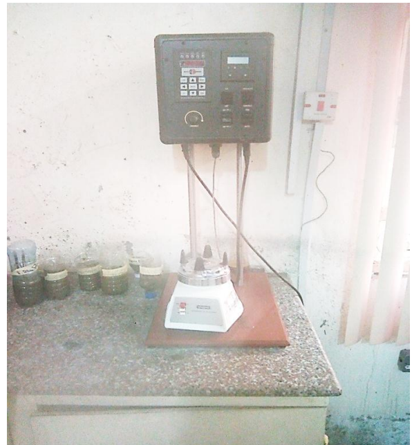
Figure 1. Warring blender for blending the cement slurry
