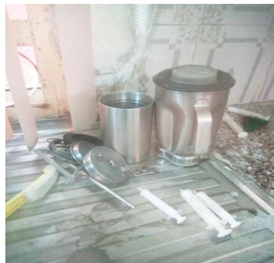
Figure 2. Blending Cup used to blend the cement slurry
