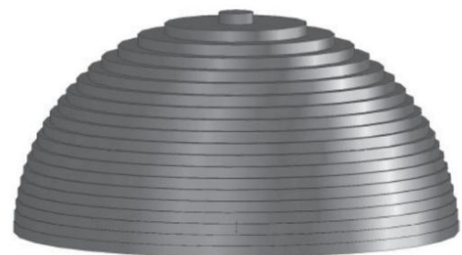
Figure 1. "Staircase" effect showed in spherical shape during Additive Manufacturing
