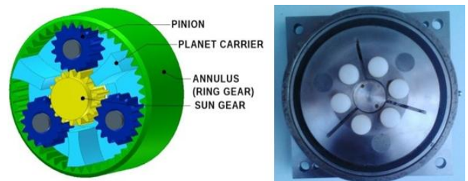
Figure 11. Planetary gearbox, on the left description of the components source: http://commons.wikimedia.org/wiki/File:Planetengetriebe_Prinzip.jpg on the right used planetary gear box
