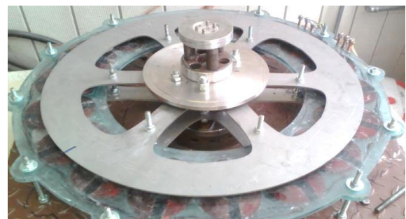
Figure 8. Axial flux PMG with 2 rotors
