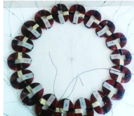
Figure 7. Arrangement of coils in the stator.
