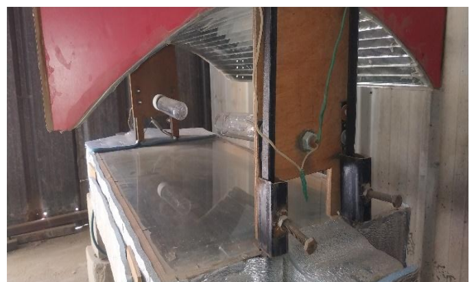
Figure 5. The constructed Simulator to be used in indoor tests of solar heaters
