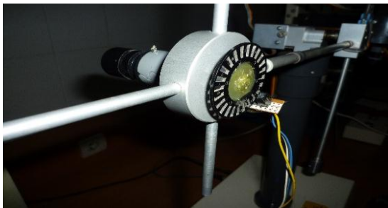
Figure 6. External incremental encoder & Optocoupler
