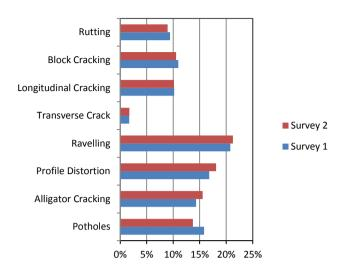
Figure 2. Comparison of Percentage of Road Damage
