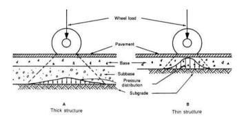
Figure 1. Distribution of Vehicle Wheel Loads
