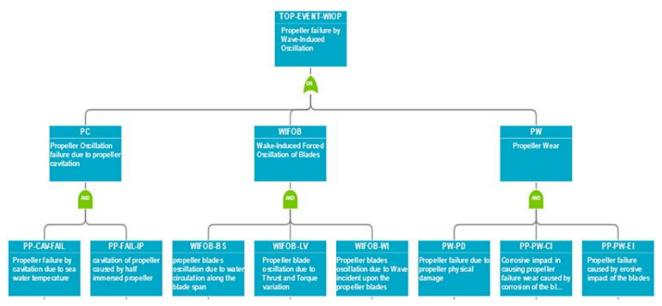
Figure 4. Fault tree analysis of propeller failure
