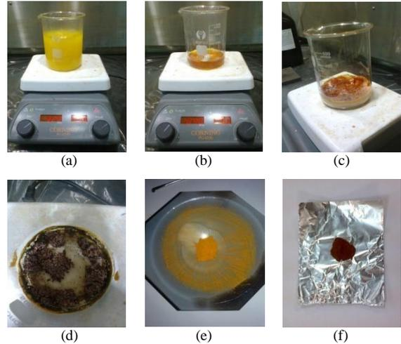
Figure 3. Synthesis steps a) mixing raw materials into deionized water, b) formation of sol, c) formation of gel, d) precursor xerogel, e) ground xerogel, f) annealed BiFeO<sub>3</sub> powder.
