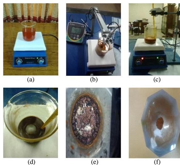
Figure 1. Synthesis steps a) Dissolving components with 4hours continuous stirring b) Solution after pH control c) Solution during heating at about  $70^\circ\text{C}$  to  $80^\circ\text{C}$  d) Onset of a thin gel like layer e) Dried gel after oven heating f) After final grinding.
