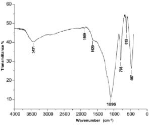
Figure 1. Infrared spectrum of an RHA sample [2].
