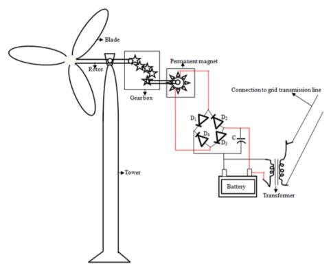
Figure 1. Wind energy conversion components
