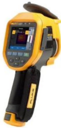
Figure 4. Thermal camera (Fluke Ti450 Pro; www.fluke.com )
